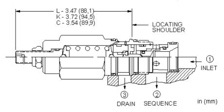
Direct-acting sequence valves will supply a secondary circuit with flow once the pressure at the inlet (port 1) has exceeded the valve setting. The pressure setting of a sequence valve controls the pressure at port 1 relative to the pressure at the drain (port 3).
