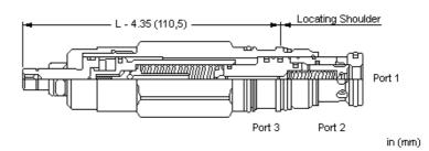
Pilot-operated, anti shock sequence cartridges limit maximum system pressure and also limit the rate of pressure rise. The valve opens and then ramps closed at a constant speed, independent of settings and flows. The adjust screw determines the maximum (relief) setting and the minimum (threshold) setting.
