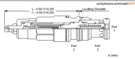
Pilot-operated, anti shock relief cartridges limit maximum system pressure and also limit the rate of pressure rise. The valve opens and then ramps closed at a constant speed, independent of settings and flows. The adjust screw determines the maximum (relief) setting and the minimum (threshold) setting.
