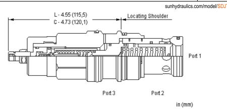
Pilot-operated, anti shock sequence cartridges limit maximum system pressure and also limit the rate of pressure rise. The valve opens and then ramps closed at a constant speed, independent of settings and flows. The adjust screw determines the maximum (relief) setting and the minimum (threshold) setting.
