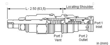
Pilot-operated, balanced poppet sequence valves will supply a secondary circuit with flow once the pressure at the inlet (port 1) has exceeded the valve setting. The pressure setting of a sequence valve controls the pressure at port 1 relative to the pressure at the drain (port 3). These valves are insensitive to back pressure at port 2 (sequence), up to the valve setting. They may be used to regulate pressure in place of 2-port relief valves if there is pressure in the return line.
