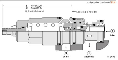
Direct-acting sequence valves with reverse-flow check will supply a secondary circuit with flow once the pressure at the inlet (port 1) has exceeded the valve setting. Additionally, these valves incorporate an integral check valve to provide reverse flow from port 2 (sequence) to port 1 (inlet). The pressure setting of a sequence valve controls the pressure at port 1 relative to the pressure at the drain (port 3).
