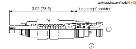
Atmospherically referenced, direct-acting sequence valves will supply a secondary circuit with flow once the pressure at the inlet (port 1) has exceeded the valve setting. The pressure setting of this sequence valve controls the pressure at port 1 relative to the atmospheric vent.
