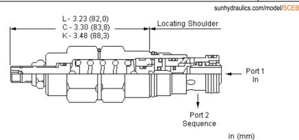
Atmospherically referenced, direct-acting sequence valves with reverse-flow check will supply a secondary circuit with flow once the pressure at the inlet (port 1) has exceeded the valve setting. Additionally, these valves incorporate an integral check valve to provide reverse flow from port 2 (sequence) to port 1 (inlet). The pressure setting of this sequence valve controls the pressure at port 1 relative to the atmospheric vent.
